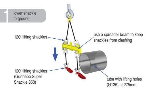
attach auxiliary lifting chains for horizontal lift
