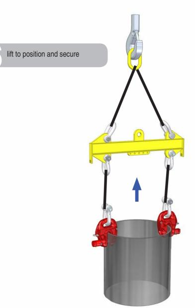
release pin and lift shackles away from tube, return to frame.
