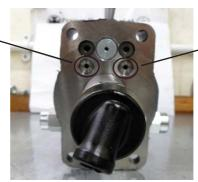
ADJUSTABLE RELIEF VALVE, PORT B (ENGAGE PIN) 100 PSI
