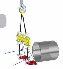
lift shackles and offer upto pile, align pin with holes in tube and engage pin
