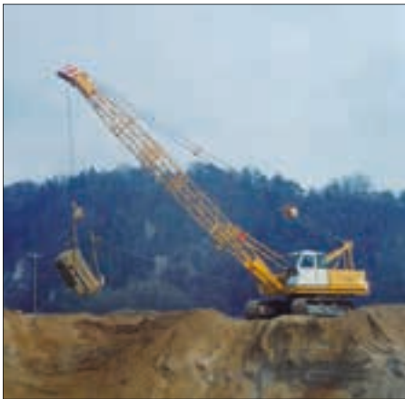
1969: First full hydraulic duty cycle crawler crane worldwide, SK 15
