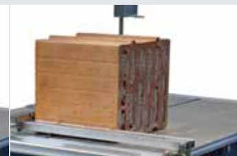
Mineral wool filled porous brick
