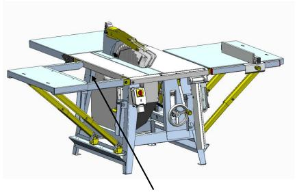
To use the cross cutting device the table insert is to remove.
