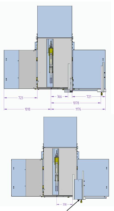
A spacer plate is required for the seamless transition from the machine table to the right table extension.
